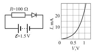
The nonlinear element is a diode with the I(V) characteristic shown.
