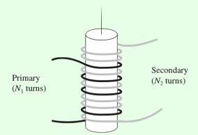
The "primary" coil has  $N_1$  turns and the secondary has  $N_2$ . If the current I in the primary is changing, show that the emf  $\mathcal{E}_2$  in the secondary obeys
