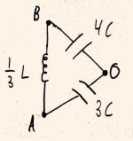
This is now a simple LC circuit with  $L_{\text{eff}} = (1/3)L$  and  $C_{\text{eff}} = (12/7)C$ , giving the final resonant frequency  $\omega_3 = \sqrt{7/4LC}$ .
