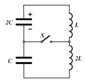
The capacitor with capacitance 2C is given a charge  $q_0$ , and immediately begins to discharge. At the moment when the current through the inductors reaches its maximum value, the switch S is closed. Find the maximum current through the switch thereafter.
