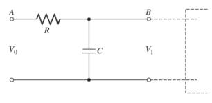
This circuit is the most primitive of "low-pass" filters.
