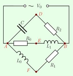
The voltage difference between D and E has amplitude  $V_{DE} = 7$  V. Similarly,  $V_{DF} = 15$  V and  $V_{EF} = 20$  V. What is the magnitude of  $V_0$ ?
