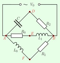
The voltage difference between D and E has amplitude  $V_{DE} = 7 \,\text{V}$ . Similarly,  $V_{DF} = 15 \,\text{V}$  and  $V_{\text{EF}} = 20 \,\text{V}$ . What is the magnitude of  $V_0$ ?
