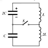
The capacitor with capacitance 2C is given a charge  $q_0$ , and immediately begins to discharge. At the moment when the current through the inductors reaches its maximum value, the switch S is closed. Find the maximum current through the switch thereafter.
