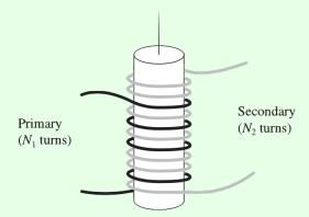
The "primary" coil has  $N_1$  turns and the secondary has  $N_2$ . If the current I in the primary is changing, show that the emf  $\mathcal{E}_2$  in the secondary obeys
