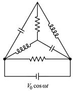
The capacitors have capacitance C, the inductors have inductance L, and the resistors have resistance  $R = \sqrt{L/C}$ . Furthermore, the driving frequency is  $\omega = 1/\sqrt{LC}$ . Find the amplitude of the total current through the circuit.
