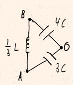
This is now a simple LC circuit with  $L_{\text{eff}} = (1/3)L$  and  $C_{\text{eff}} = (12/7)C$ , giving the final resonant frequency  $\omega_3 = \sqrt{7/4LC}$ .
