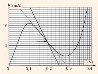
By plotting  $\mathcal{E} - IR$  on the graph above, we find  $I_0$  at the intersection. Now consider the effect of applying the signal voltage, which changes the current by  $\Delta I$ ,
