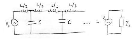
(b) The diagram below shows two adjacent sections of the ladder.
