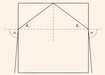
Assuming  $n > \sqrt{2}$ , we then have  $\theta_r < 45^\circ$ , and then the laser internally reflects when it hits the top surface of the cube. It exits in the opposite direction it came in.
