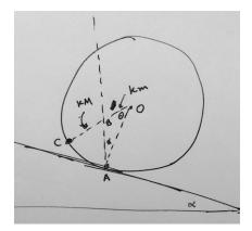
We see that the center of mass of the cylinder-block system must be right above the contact point A. Now, we see that the CM is at B where CB/BO = M/m. Thus, OA = OB + OC = k(m + M), so by the law of sines on OAB, we have
