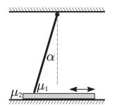
Underneath, a thin board is being dragged on the floor. The coefficient of (static and kinetic) friction is  $\mu_1$  between the board and rod, and  $\mu_2$  between the board and floor. The rod is meant to stop the board from being dragged to the right, no matter how hard or how quickly it is pulled. Is this possible? If so, what are the conditions on the parameters that allow this to occur?
