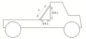
There is no friction between the top of the board and the vertical surface of the truck. The coefficient of static friction between the bottom of the board and the horizontal surface of the truck is  $\mu_s = 0.5$ . The truck always moves in the forward direction.
