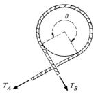
The rope is wrapped around a fixed drum with coefficient of friction  $\mu$ , usually for several turns. The load on the rope pulls it with a force  $T_A$ . Ignore gravity.
