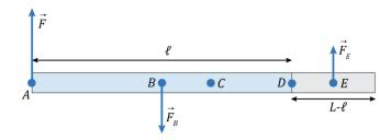
The figure above shows a top-down view of the bar. Just before slipping, friction has the maximum possible magnitude everywhere, and points either directly against or directly along the force you exert. Using the variables defined in the figure, just barely balancing forces and torques simultaneously gives
