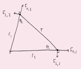
Consider force balance on the first marked vertex. The tension in the side of length  $r_2$  takes whatever value is necessary to balance the horizontal force on the vertex, while the tension T in the other side has to balance the vertical force. Thus,
