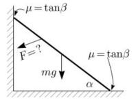
What is the minimum additional force F needed to keep the rod static?
