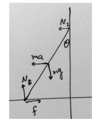
Force balance gives mg = N and  $N_2 + ma = f$ , and torque balance gives
