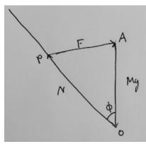
We see that the magnitude of N varies as P varies along the line  $\ell$  which is the line at angle  $\phi$  to AO, and the magnitude of F is AP. AP is minimized when P is the foot of the altitude from A to  $\ell$ , so we see
