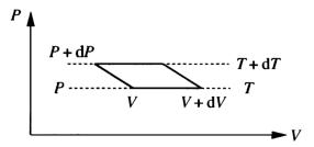
By equating the efficiency of this cycle to the Carnot efficiency, find  $(\partial U/\partial V)|_T$ .
