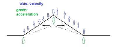
To derive the acceleration, you can think about how the velocity profile has to change as the string moves, or you can think about how it comes about from the tension in the string. In general, the net force depends on the concavity  $\partial^2 y/\partial x^2$  of the string. In this case, it's only nonzero at the three kinks.
