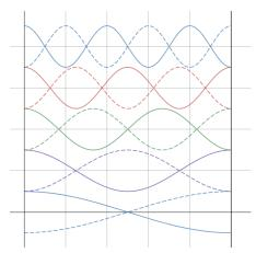
Technically, while the boundary conditions in part (a) required  $n \ge 1$ , here we can actually take  $n \ge 0$ . The n = 0 solution just corresponds to the whole string being moved up or down and staying there, with zero frequency. But this trivial solution is not typically called a "standing wave", so it's conventional to say the lowest frequency is at n = 1.
