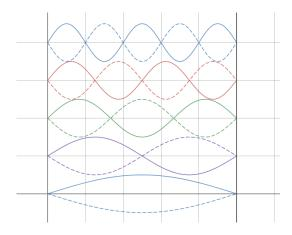
(b) We can replace the sine with a cosine in the above solution (so integrating or differentiating the above solution with respect to x gets the solutions to this problem). Thus the frequencies are the same,  $\omega_n = \pi v n/L$ , and the waves look like this:
