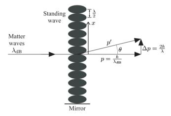
Suppose the frequency of the light is close enough to an atomic transition to cause significant interaction, but not close enough to make spontaneous emissions important. Then we can think of the light as just shifting the atomic energy levels, depending on the local field intensity. This leads to a pattern of phase shifts in the matter wave with spatial period  $d = \lambda/2$ , which means the grating diffracts matter waves at angles obeying
