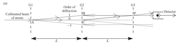
The diffraction gratings here are identical, and spaced so that the slits of one fall at the maxima of the previous one. As a result, atoms can propagate from A to P via either B or C. This is precisely the form of a Mach–Zehnder interferometer.
