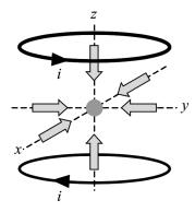
The two current loops create a magnetic quadrupole field near the origin, where the magnetic field vanishes.
