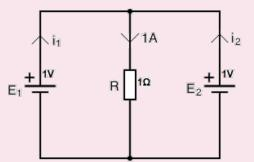
For example, in the above circuit, Kirchoff's rules don't determine the currents; they only say that  $i_1 + i_2 = 1$  A. If the emfs of the batteries were different, the situation would be even worse: the equations would be contradictory, with no solution at all! In real life, this is avoided because all batteries have some internal resistance. Adding such a resistance to each battery, no matter how small, resolves the problem and gives a unique solution.
