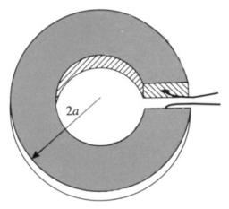
Since the washer has an irregular shape, the current distribution inside it is complicated: it spreads out from the first wire, goes around the washer, and converges into the second wire. However, the situation is simpler if we glue a perfectly conducting square plate, of side length a, to each exposed face. Find the resistance in this case.
