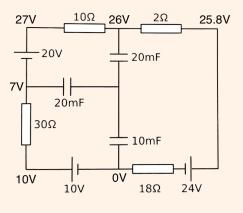
To finish the problem, we need to know the voltage  $V_0$  of the central node, so we need one more equation. That equation is charge conservation. We note that the central part of the circuit, containing the inner plates of the three capacitors, begins uncharged and is not directly connected to anything else, so it must remain uncharged. (Charge can't move through a capacitor!) Suppressing units, this means
