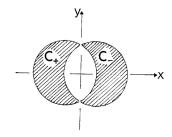
The current in each conductor is uniformly distributed. Find the magnetic field in the space between the conductors.
