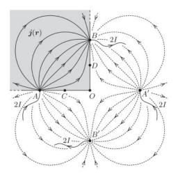
We have a new current source and sink respectively at the reflections of A and B in O. The current sources and sinks all have magnitude 2I, rather than I, because only half of the currents at A and B actually enter and exit the physical plate, shaded in gray.
