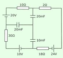
After a long time, what is the charge stored on the 10 mF capacitor?
