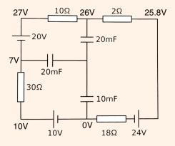
To finish the problem, we need to know the voltage  $V_0$  of the central node, so we need one more equation. That equation is charge conservation. We note that the central part of the circuit, containing the inner plates of the three capacitors, begins uncharged and is not directly connected to anything else, so it must remain uncharged. (Charge can't move through a capacitor!) Suppressing units, this means
