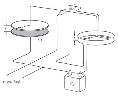
The force between capacitor plates is balanced against the force between parallel wires carrying current in the same direction. A voltage alternating sinusoidally with angular frequency  $\omega$  is applied to the parallel-plate capacitor  $C_1$  and also to the capacitor  $C_2$ , and the current is equal to the current through the rings. Assume that  $s \ll a$  and  $h \ll b$ .
