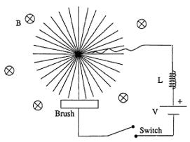
A battery with voltage V feeds current through an inductor L, into the axle, through the spoke, to the brush. There is a uniform magnetic field **B** pointing into the plane of the paper. At time t = 0 the switch is closed.
