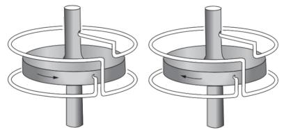
It has only two essential parts. One part is a solid metal disk and axle which can be driven in rotation. The other is a two-turn "coil" which is stationary but is connected by sliding contacts, or "brushes", to the axle and to the rim of the revolving disk.
