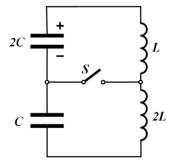
The capacitor with capacitance 2C is given a charge  $q_0$ , and immediately begins to discharge. At the moment when the current through the inductors reaches its maximum value, the switch S is closed. Find the maximum current through the switch thereafter.
