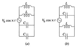
In each case, find the amplitude of the current drawn from the source as a function of  $\omega/\omega_0$ , where  $\omega_0 = 1/\sqrt{LC}$ .
