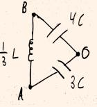
This is now a simple *LC* circuit with  $L_{\text{eff}} = (1/3)L$  and  $C_{\text{eff}} = (12/7)C$ , giving the final resonant angular frequency  $\omega_3 = \sqrt{7/4LC}$ .
