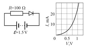
The nonlinear element is a diode with the I(V) characteristic shown.
