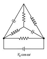
The capacitors have capacitance C, the inductors have inductance L, and the resistors have resistance  $R = \sqrt{L/C}$ . Furthermore, the driving angular frequency is  $\omega = 1/\sqrt{LC}$ . Find the amplitude of the total current through the circuit.
