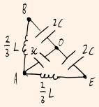
We now apply the same procedure between points B and E. This circuit is again a balanced Wheatstone bridge, so O and A are at the same voltage. We then have a simple LC circuit with  $L_{\text{eff}} = (4/3)L$  and  $C_{\text{eff}} = C$ , giving  $\omega_2 = \sqrt{3/4LC}$ .
