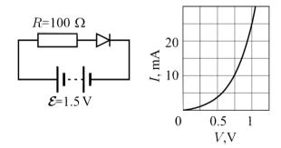
The nonlinear element is a diode with the I(V) characteristic shown.
