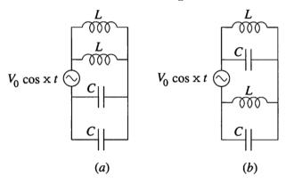
In each case, find the amplitude of the current drawn from the source as a function of  $\omega/\omega_0$ , where  $\omega_0 = 1/\sqrt{LC}$ .
