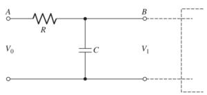
This circuit is the most primitive of "low-pass" filters.
