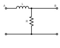
(c) Here's one possible answer. You could also take the low-pass filter in part (a) and switch the locations of the capacitor and resistor.
