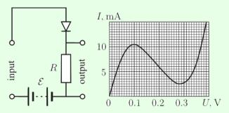
Here,  $R = 10 \Omega$  and  $\mathcal{E} = 0.25 \,\mathrm{V}$ . If a small signal voltage  $V_{\mathrm{in}}(t)$  is applied across the input, then an amplified and shifted version of the signal appears across the output. Find the amplification factor.
