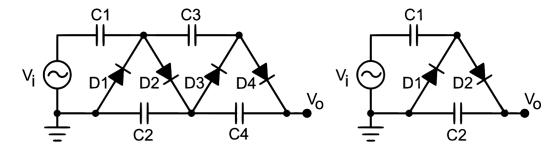
The four capacitors begin uncharged, and all have capacitance C. All four diodes are ideal. The voltage  $V_i(t)$  alternates between V and -V. The output voltage is  $V_0$ .
