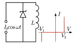
The inductance L of the inductor is such that  $L\omega I_0 \gg V_1, V_2$  where  $V_1$  and  $V_2$  are the breakdown voltages, and  $V_1 > V_2$ . The I(V) characteristic of the Zener diode is shown above. Assume that a long time has passed since the current source was first turned on.
