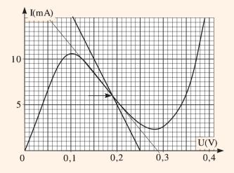
By plotting  $\mathcal{E} - IR$  on the graph above, we find  $I_0$  at the intersection. (Notice the x-axis label: it is common to write a decimal point as a comma in Eastern Europe.) Now consider the effect of applying the signal voltage, which changes the current by  $\Delta I$ ,
