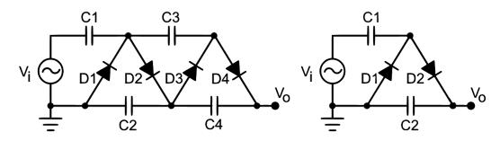
The four capacitors begin uncharged, and all have capacitance C. All four diodes are ideal. The voltage  $V_i(t)$  alternates between V and -V. The output voltage is  $V_0$ .
