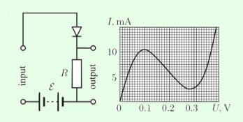
Here,  $R = 10 \Omega$  and  $\mathcal{E} = 0.25 \text{ V}$ . If a small signal voltage  $V_{\text{in}}(t)$  is applied across the input, then an amplified and shifted version of the signal appears across the output. Find the amplification factor.
