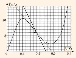
By plotting  $\mathcal{E} - IR$  on the graph above, we find  $I_0$  at the intersection. (Notice the x-axis label: it is common to write a decimal point as a comma in Eastern Europe.) Now consider the effect of applying the signal voltage, which changes the current by  $\Delta I$ ,
