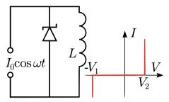
The inductance L of the inductor is such that  $L\omega I_0 \gg V_1, V_2$  where  $V_1$  and  $V_2$  are the breakdown voltages, and  $V_1 > V_2$ . The I(V) characteristic of the Zener diode is shown above. Assume that a long time has passed since the current source was first turned on.
