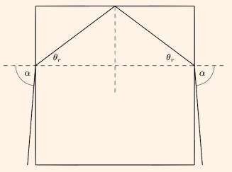
Assuming  $n > \sqrt{2}$ , we then have  $\theta_r < 45^{\circ}$ , and then the laser internally reflects when it hits the top surface of the cube. It exits in the opposite direction it came in.
