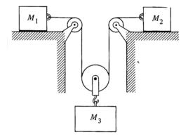
The coefficient of friction between the masses and the horizontal surfaces is  $\mu$ . Show that the tension in the rope is
