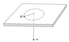
The system is set up so that the mass M moves in a circle of radius r, while the mass m remains still. Show that this motion is stable with respect to small changes in r, and find the angular frequency of small oscillations.
