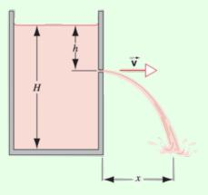
Find the distance x from the foot of the wall at which the stream strikes the floor.
