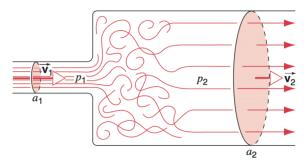
The jet will mix with the surrounding fluid, forming a turbulent region where the pressure is approximately  $p_1$ . Further to the right, the flow becomes almost uniform again, with average speed  $v_2$  and pressure  $p_2$ .
