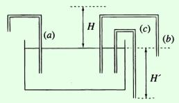
Note that H' > H. For which tubes, if any, does water flow out of the other end?
