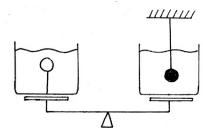
In the left-hand vessel you suspend a very light ping-pong ball on a thin, light wire attached to the base of the vessel. In the right-hand vessel you suspend a ping-pong ball filled with lead, again by a light thin wire. Do the scales stay level, go down on the left, or go down on the right?
