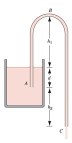
The tube must initially be filled, but once this has been done the liquid will flow until its level drops below the tube opening at A. The liquid has density  $\rho$  and negligible viscosity.
