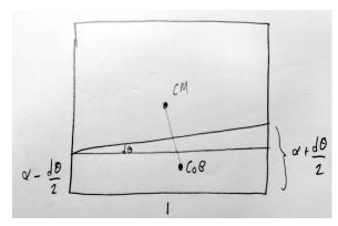
The fraction of the log submerged is  $\alpha$ . To compute the coordinates of the center of buoyancy we split it into two pieces as shown above. Then
