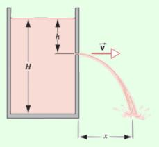
Find the distance x from the foot of the wall at which the stream strikes the floor.
