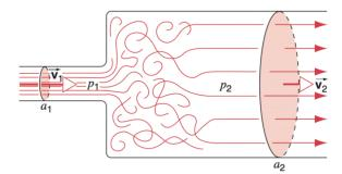
The jet will mix with the surrounding fluid and, after the turbulent mixing, will flow on almost uniformly with an average speed  $v_2$ .
