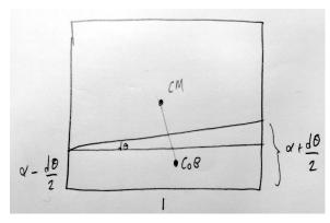
The fraction of the log submerged is  $\alpha = \rho_{\log}/\rho_{\text{water}}$ . To compute the coordinates of the center of buoyancy we split it into two pieces as shown above. Then
