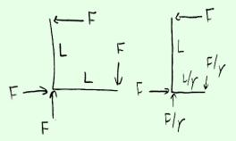
In a frame where the lever moves to the right with speed v, one of the lever arms will be contracted to  $L/\gamma$ , as shown at right. In addition, by the results of problem 18, the vertical external forces will be redshifted to  $F/\gamma$ . This implies a net torque of
