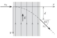
When the electron leaves the field, its velocity makes an angle  $45^{\circ}$  with its initial direction.
