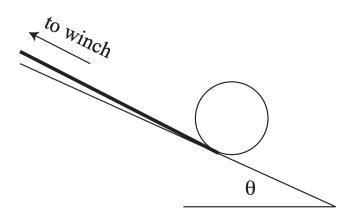
The winch has radius  $r_w$  and can be set to turn a fixed number of turns  $n_t$  with a constant torque  $\tau$ , i.e.  $\tau/r_w$  is the tension in the winching string. The can is initially held stationary, and is then released. It is observed that the winch stops turning after a time t. Neglect friction between the can and slope and treat the string as massless.
