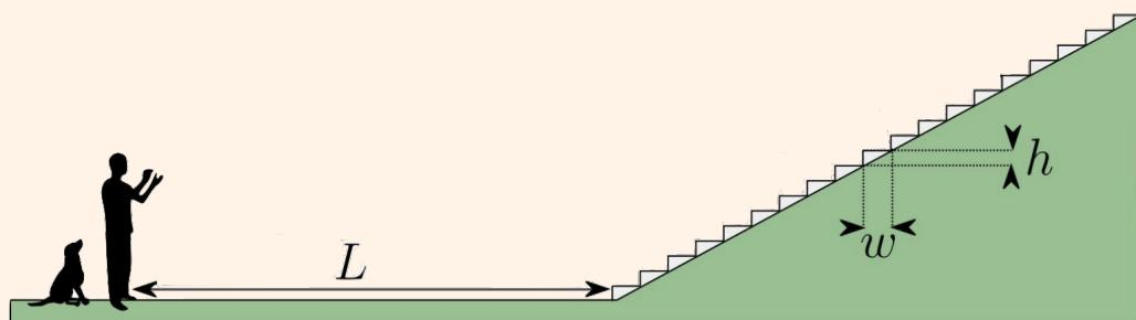
The key is that each clap reflects off a stair individually. When the echoes arrive back at the listener, they arrive quickly enough to be heard as a pitch.
