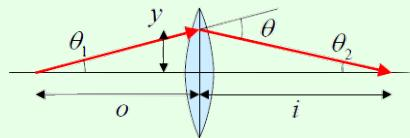
An image is formed a distance  $i$  in front of the lens. How are  $o$ ,  $i$ , and  $f$  related?
