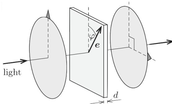
If the system is illuminated with light of wavelength  $\lambda$ , give a value for  $d$  and orientation of  $\mathbf{e}$  that maximizes the transmitted light.
