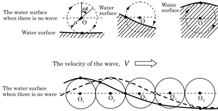
(a) Consider the frame of reference moving to the right with velocity  $v$ . In this frame, the surface of the water is completely stationary, while molecules travel along the surface. Consider a small parcel of water which travels from a valley to a peak. By applying conservation of energy, derive a relationship between  $v$ ,  $\omega$ , and  $g$ .
