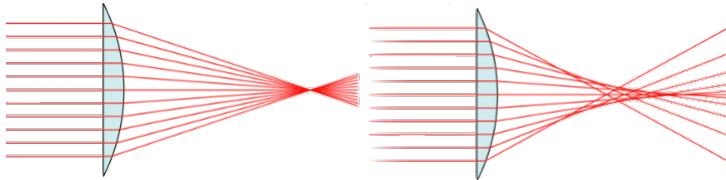
You should find that  $x(y)$  is not an arc of a circle, which implies that a spherical lens will fail to focus all incoming horizontal light to a point. Instead, we will get spherical aberration, as shown at right above. However, most lenses are spherical because it's easier to make them that way.
