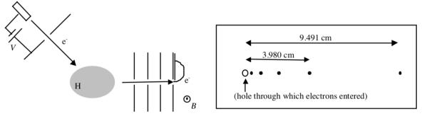
When the film is developed, a series of spots is observed. The distances between the hole and the two most distant spots are measured. You may assume that the film is large enough to have intercepted all of the electrons, i.e. that there are no spots farther from the hole than those shown. The number of spots shown is not necessarily accurate.
