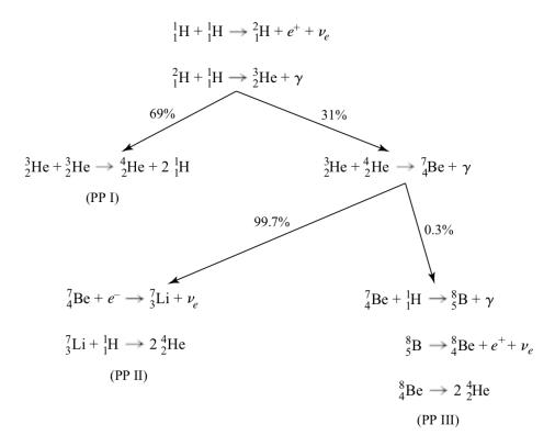
The first step is one of the slowest, because it is a weak process. The proton-proton chain is the dominant fusion mechanism in the Sun, and near the core temperatures of  $T_6 \approx 15$ , the temperature scaling is  $\beta \approx 4$ , which is relatively weak.
